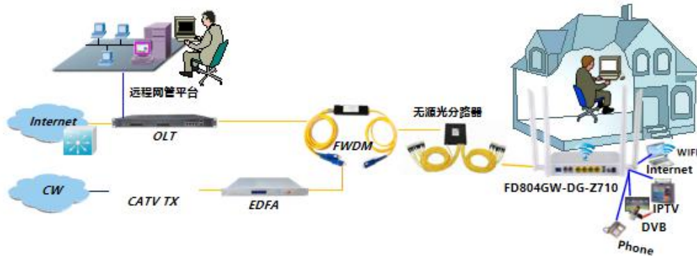
Figure: FD804GW-DAG-Z710 ONU Application Diagram
